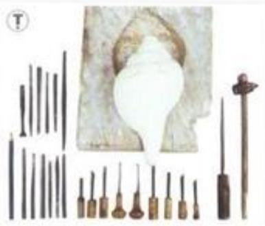
Key equipment used for conch carvings are file, chisels, hammer, grinder etc. The chisels are used in different sizes depending on the detailing and intricacies of the pattern.
